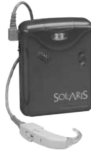
A body-worn receiver with a cord to coupling adapter and hearing aid
